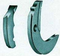
Fitting Inserted Points. After inserting a set of points, the shanks should be carefully examined to see that none project on either side of the plate. They should be exactly on the center. This is of special importance when a narrow kerf is desired, for if the shank is allowed to project a little on one side when the kerf is narrow it would be likely to rub against the side of the cut and cause trouble.
