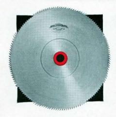
Mitre Saws are ground tapering to the collar, to run without set and provide ample clearance. They are especially adapted to smooth, clean cutting such as cabinet and cigar-box work.
