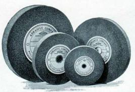
Simonds Abrasive grinding wheels do a variety of work in the machine shop. Sharpening tools such as twist drills, milling cutters, reamers and lathe tools are some of the important jobs where a medium grained wheel is generally used. Fine grain wheels adapt themselves to the sharpening of delicate edged tools and in places where a good finish is desired. Cleaning
