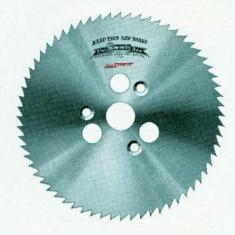
Simonds Electrotype Saws are made in sizes from 5 to 10 inches in diameter to fit any type of trimmer machine. The teeth are set and filed or swaged or the saws are concave ground for clearance. Electrotype Saws are made with pitched to center teeth, ½ to ½ inch space. Formed teeth are also furnished.
