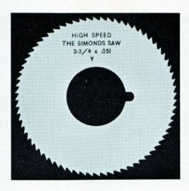
Screw Slotters are used mostly for cutting slots in screw heads, and are made with fine teeth for the reason that the heads on screws vary from  $\frac{1}{16}$  inch to 1 inch in diameter. They are made with fine teeth to prevent shelling of teeth which might occur if the space between the teeth was more than the diameter of small screw heads, such as  $\frac{1}{16}$  inch.
