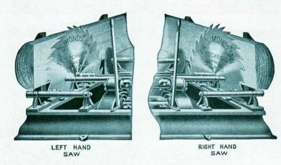
N. B.—Standing in front of a circular saw (with the saw revolving towards you), if the log passes to the right of the saw it is a Right Hand Saw; if to the left, a Left Hand Saw, as shown above.
