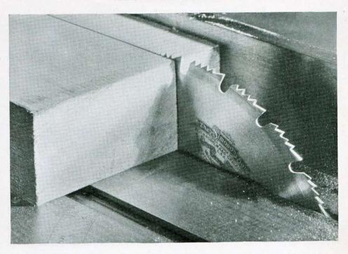
This saw will work successfully in soft or hard wood, whether ripping, cutting off, or mitering and will stand fast hand feed without rubbing or overheating.
