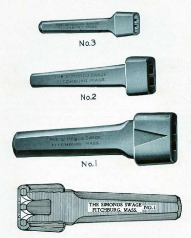
This sectional view shows the construction of the Simonds Swage. Jaw No. 1 spreads or shapes the point of the tooth. Jaw No. 2 squares up the cutting edge and gives body to the swaged point.
